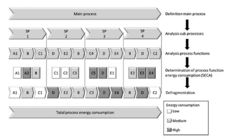
Fig. 8. Energy monitoring process (Source: created by the authors)
