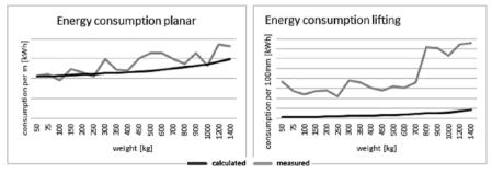
Fig. 5. Deviation of process energy consumption in planar handling and lifting (Source: created by the authors)
